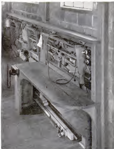
Clamping work between the vise and a solid backing of "four by fours." Right, view showing end of cabinets and angle brace under the bench top
